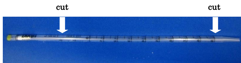
Fig. 4 How to cut out a scaled part from a pipette
